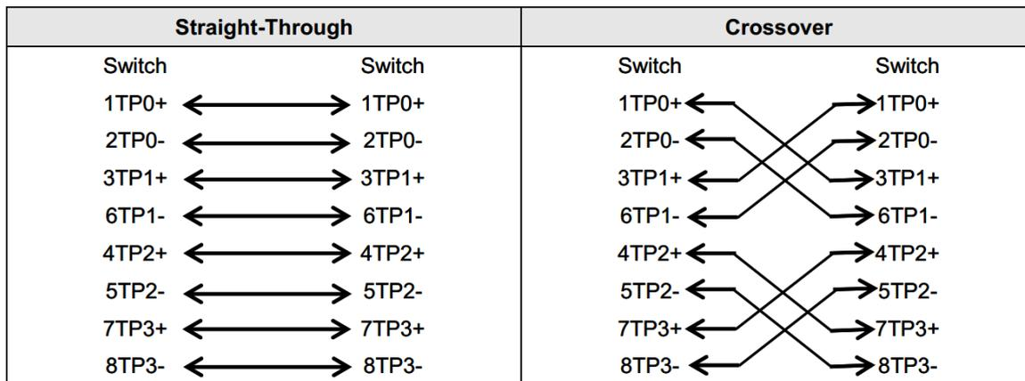
10BASE-T uses Category 3, 4, 5 100-ohm UTP/STP and 1000BASE-T uses Category 5 100-ohm UTP/STP for connections. Both support a maximum length of 100 meters. Table A-1 shows 100BASE-TX/10BASE-T pin assignments.
