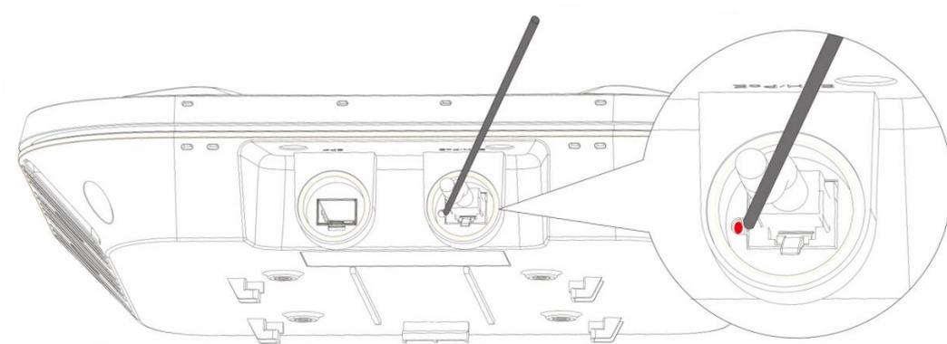
**i** Before pressing the reset button, please remove the waterproof joint first. Refer to the Chapter 3.5 Connecting Cables for more information.
